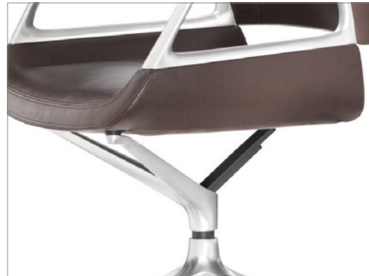
Elastic connecting elements at the front and a springy brace at the rear mean the seat adapts forward and backward to the body's center of gravity.
